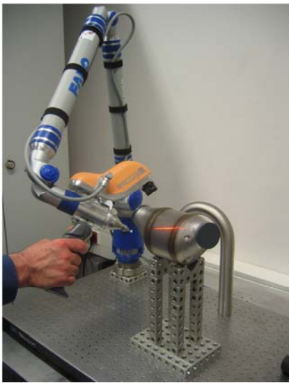
Articulated measuring arm with split beam sensor
